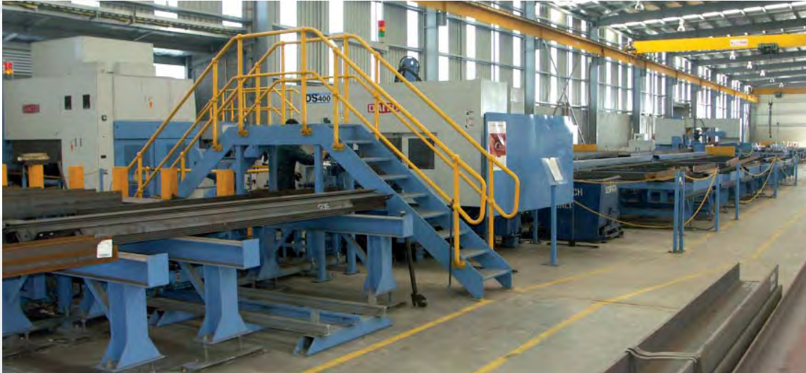
← LEFT Dual saw/drill beamline includes in-parallel layout for maximum output. ↓ BELOW CNC Automated Plasma Notching Robot.
